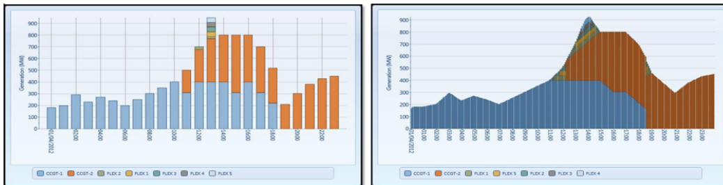
FIGURE 16 Dispatch simulation results in hourly (left) and 5 minute resolution (right), with obvious differences in the operation patterns of individual generators. 22
